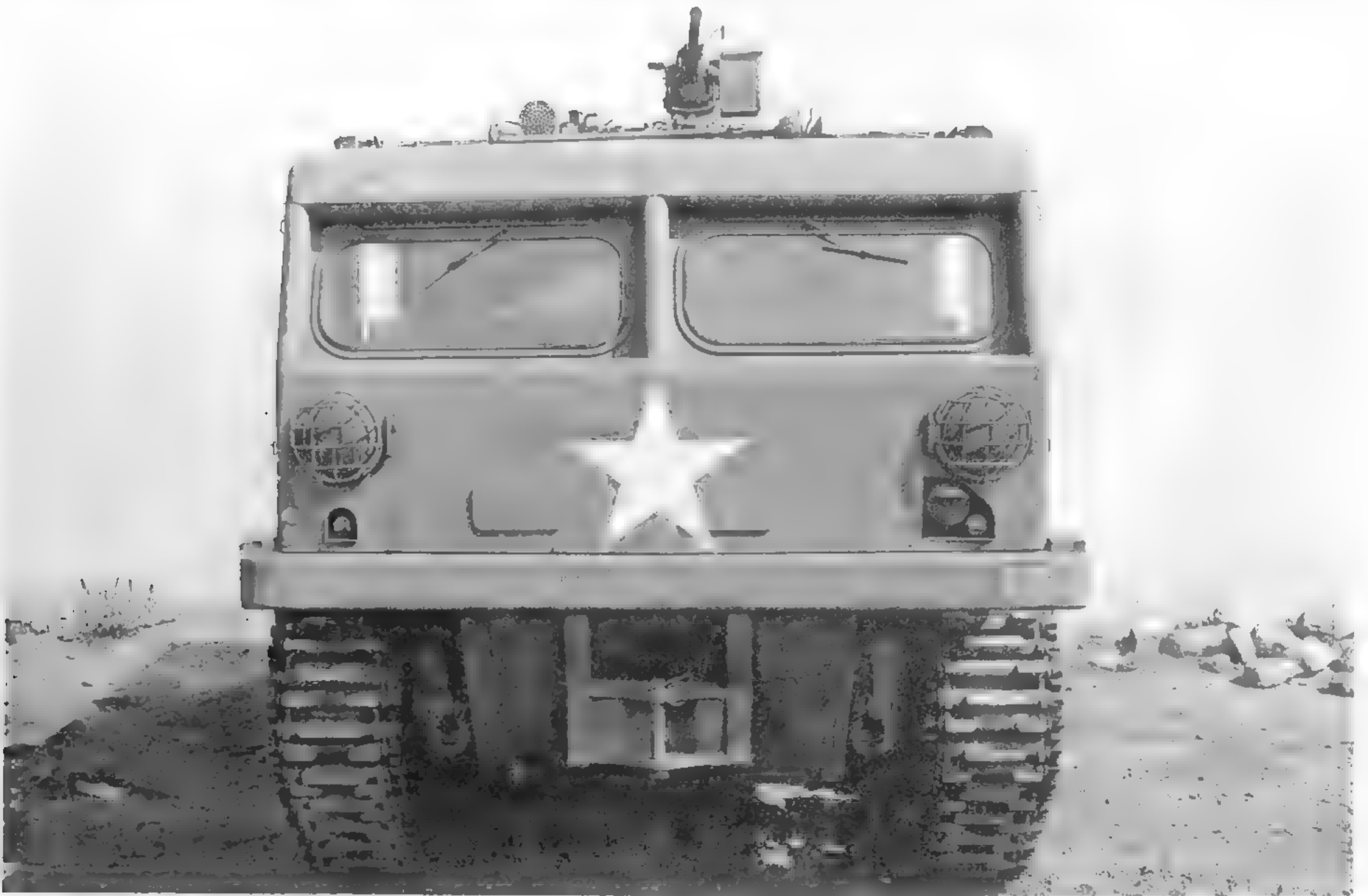
The M4 had narrower tracks and spacing than the M4A1. (U.S. Army photo)
